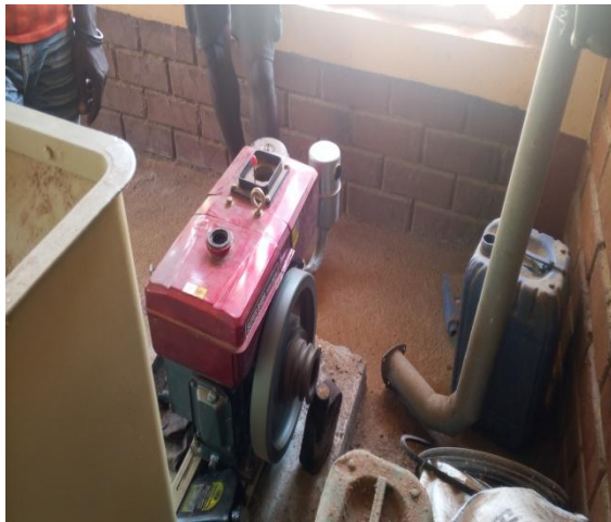
No fan belt & cover for destoner; Leakage in borehole piping (Wulanthenki, Magbema Chiefdom)
