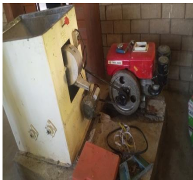
Milling machine and destoners and unmounted water tanks in Peyima (Kamara Chiefdom, Kono District)
